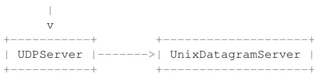
Note that `UnixDatagramServer` derives from `UDPServer`, not from `UnixStreamServer` --- the only difference between an IP and a Unix stream server is the address family, which is simply repeated in both Unix server classes.
