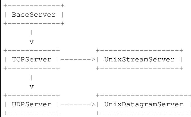
Note that `UnixDatagramServer` derives from `UDPServer`, not from `UnixStreamServer` --- the only difference between an IP and a Unix stream server is the address family, which is simply repeated in both Unix server classes.
