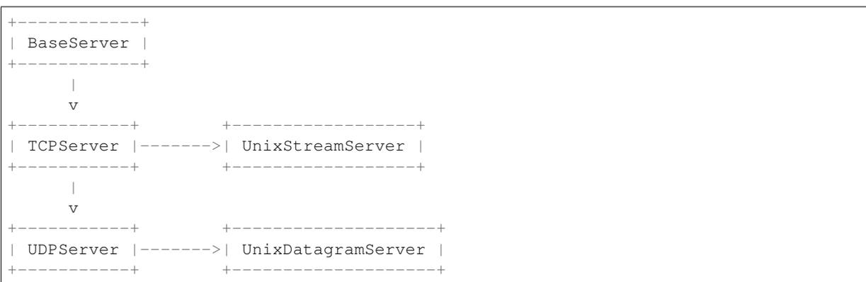
Note that *UnixDatagramServer* derives from *UDPServer*, not from *UnixStreamServer* --- the only difference between an IP and a Unix stream server is the address family, which is simply repeated in both Unix server classes.
