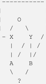
In this case, it is not possible to derive a new class C from A and B, since X precedes Y in A, but Y precedes X in B, therefore the method resolution order would be ambiguous in C.
