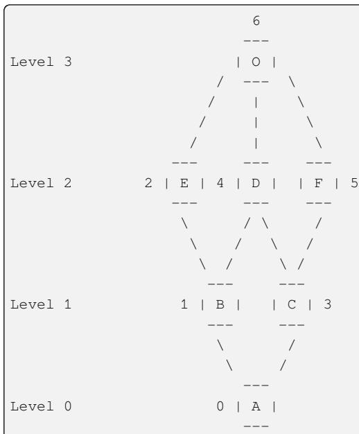
Notice that the class E, which is in the second level of the hierarchy, precedes the class C, which is in the first level of the hierarchy, i.e. E is more specialized than C, even if it is in a higher level.
