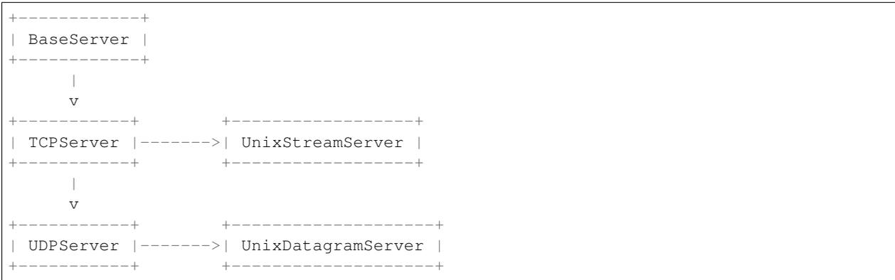
Note that *UnixDatagramServer* derives from *UDPServer*, not from *UnixStreamServer* --- the only difference between an IP and a Unix stream server is the address family, which is simply repeated in both Unix server classes.
