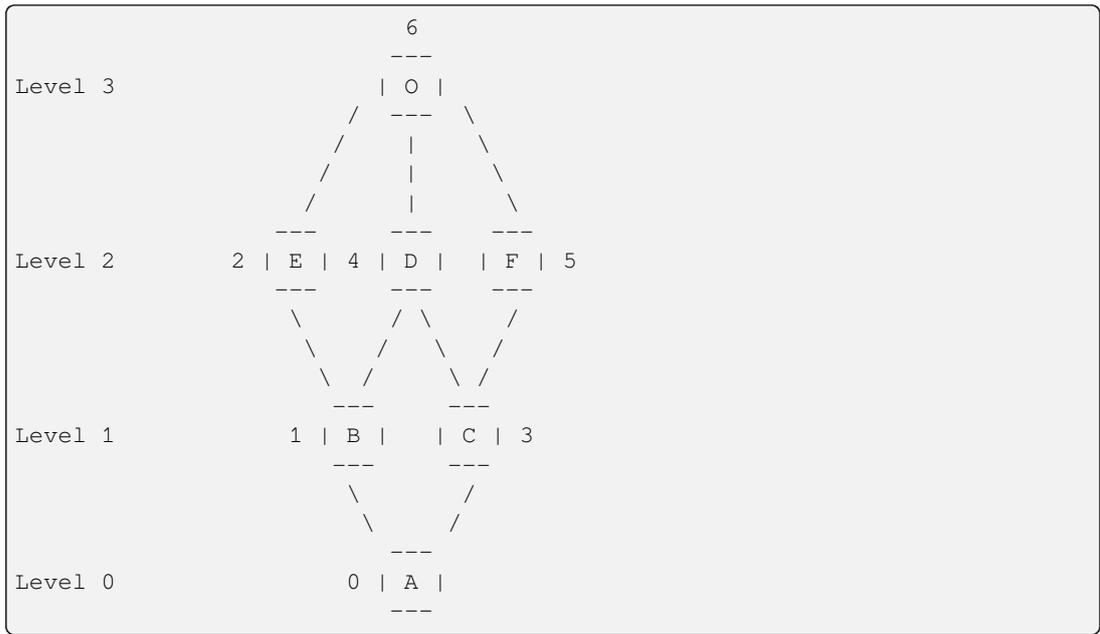
Notice that the class E, which is in the second level of the hierarchy, precedes the class C, which is in the first level of the hierarchy, i.e. E is more specialized than C, even if it is in a higher level.
