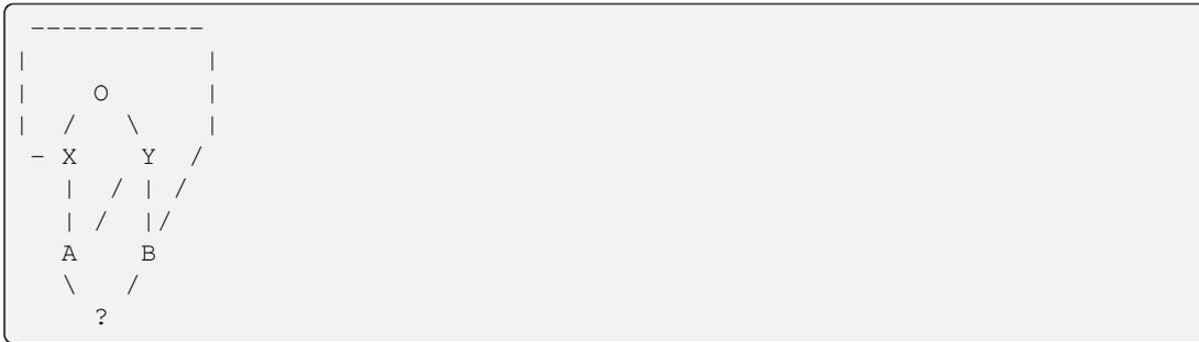
In this case, it is not possible to derive a new class C from A and B, since X precedes Y in A, but Y precedes X in B, therefore the method resolution order would be ambiguous in C.
