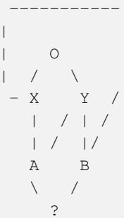
In this case, it is not possible to derive a new class C from A and B, since X precedes Y in A, but Y precedes X in B, therefore the method resolution order would be ambiguous in C.
