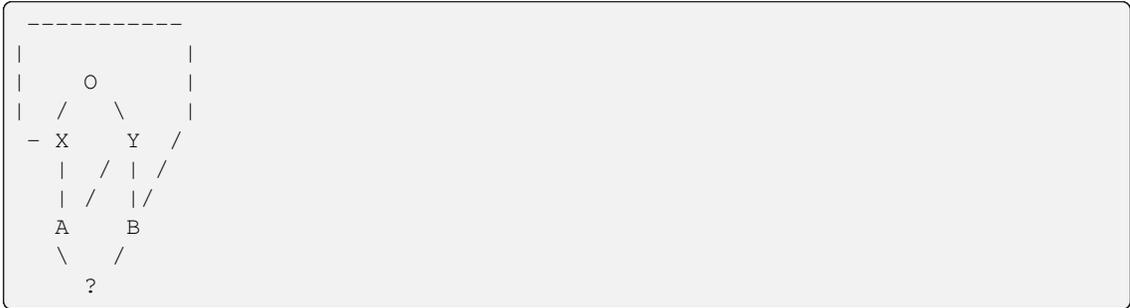
In this case, it is not possible to derive a new class C from A and B, since X precedes Y in A, but Y precedes X in B, therefore the method resolution order would be ambiguous in C.
